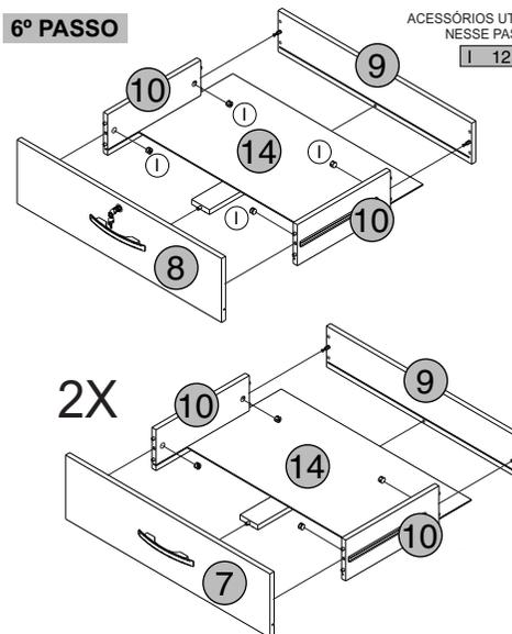
ENCAIXE O FUNDO DA GAVETA NAS LATERAIS E FIXE O CONTRAFUNDO E A FRENTE DA GAVETA NAS LATERAIS COM TAMBOR MINIFIX (I) JUNTANDO A TRAVA DA GAVETA ENTRE A FRENTE E O CONTRAFUNDO
